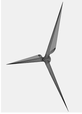
Fig. 2. A 3D model adapted from [17] and used for RCS simulations and studying the maximum, mean and median values of blade flashes. The blade lengths were scaled to 85 m.
